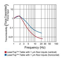
TMC Pneumatic Isolators exhibit high attenuation of both vertical and horizontal Vibration, even at the low amplitude levels typical of most laboratory floors.
